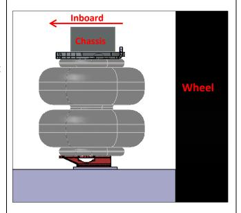
The lower bracket is mounted on the leaf spring with the tabs facing inboard.
