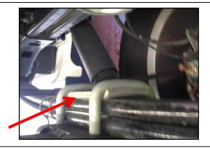
Position the assembly on top of the leaf and install the new saddle between the U-Bolts.
