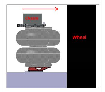
The lower bracket is mounted on the leaf spring with the tabs facing outboard.
