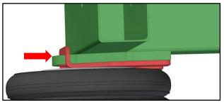
Bolt the upper air spring bracket to the Upper Chassis Bracket with the M10x1.5-30mm coach bolts, flat washers and nyloc nuts provided.
