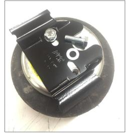
Fasten the Air Spring to the Lower Bracket. Use the M10x1.5-20mm Hex bolts and washers provided.
